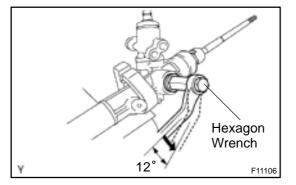
(b) Using a hexagon wrench (19 mm), torque the rack guide spring cap.
