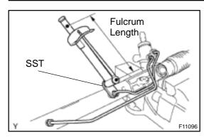
(b) Using SST, install the 2 turn pressure tubes. SST 09023–38200
